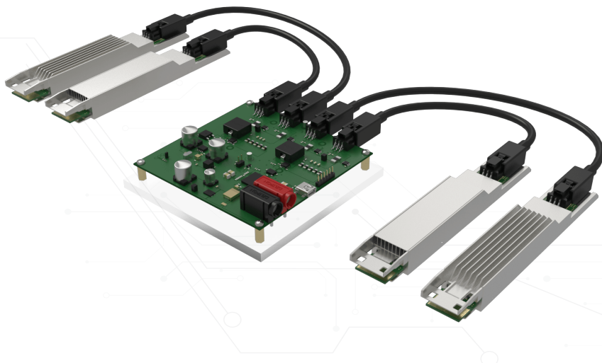
Four ML4064-XD-TL thermal loads plugged into the ML4064-XD-CNT thermal controller board
